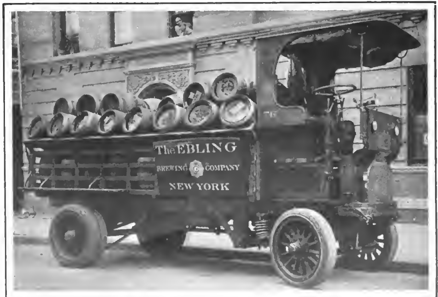
Five-ton High Cab "76" with Williams suspension, carrying 6 tons
